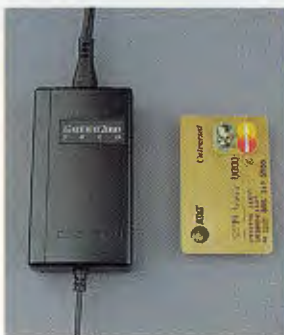
The power supply is small and light. Leaving it out of the case eliminated the need for a cooling fan.
