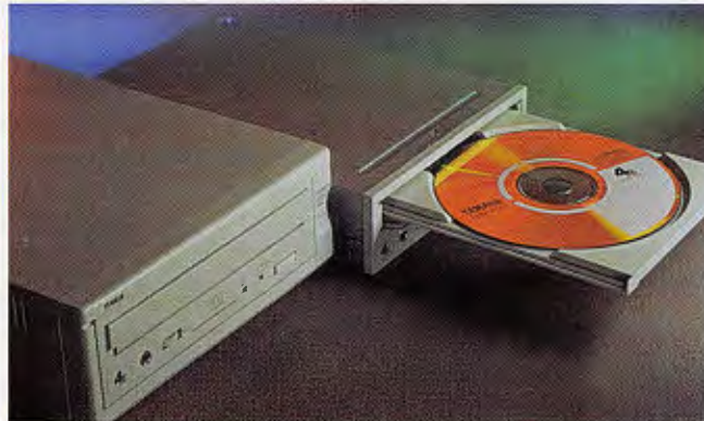
Yamaha's CDR400 will write to CD-R media at 4x speed, and read from CDs at 6x speed. Yamaha also announced it would be entering the retail channel for the first time.
